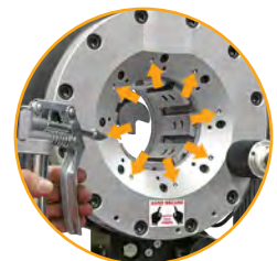
Easy grease maintenance through the 8 lubrication fittings.
