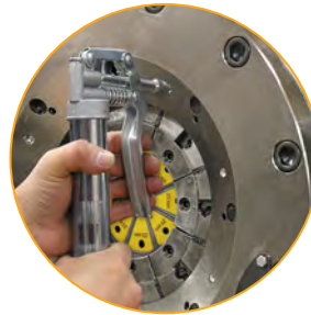
New Grease Applied on All Wear Surfaces
