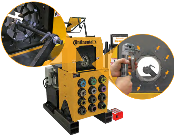
Intuitive screens lead the operator through the setup and crimping process.
