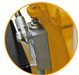
Safety Switch activates and drops pressure as soon as the lid is opened.
