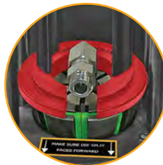
Notched pressure plate ideal when crimping 90° fittings.
