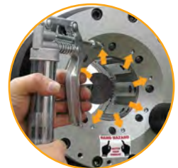
Easy grease maintenance through the 8 lubrication fittings.
