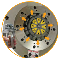
Easy grease maintenance through the 8 lubrication fittings.
