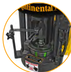
Coupling stop makes repetitive crimps faster.
