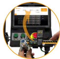
CrimplIQ™ controller supports bluetooth calipers to input crimp diameter measurements.
