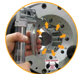
Easy grease maintenance through the 8 lubrication fittings.
